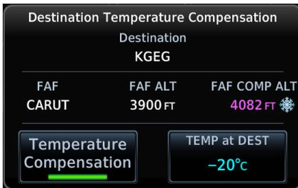
Temperature compensated approach plate altitude restrictions are shown with a corresponding snowflake icon for each adjusted altitude on the active flight plan.
