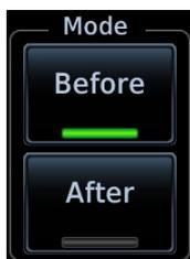
Inserting an ATK before the selected waypoint results in a negative offset value. Inserting it after results in a positive value.
