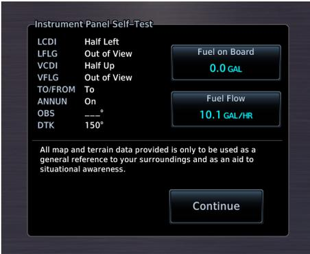
If configured, the results of all external equipment checks performed by the unit display on the Instrument Panel Self-Test page.
