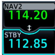
Changes in radio selection and standby frequency are reflected in the control bar.
